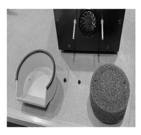
To check your filters, hold them up to a light, similar to your car air intake filter. If you cannot see light through more than 50% of the filter, replace filter element or clean it.
