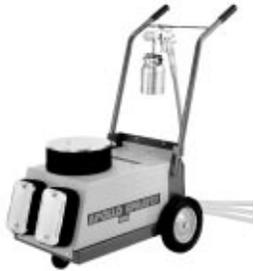
**MODEL 1100**—Dual Turbines, 3.5 - 10psi. (24 bar, 41 bar, 69 bar) 44' (13.41m) Slim-Flex™ air hose, Apollo HVLP Spray Gun. 77lbs (35kg), 110v, 60Hz, 15amps, 2.6hp. (240v, 50Hz, 7.5amps).
